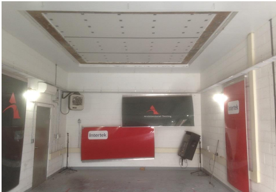
Receive Room View of Test Specimen Installation
