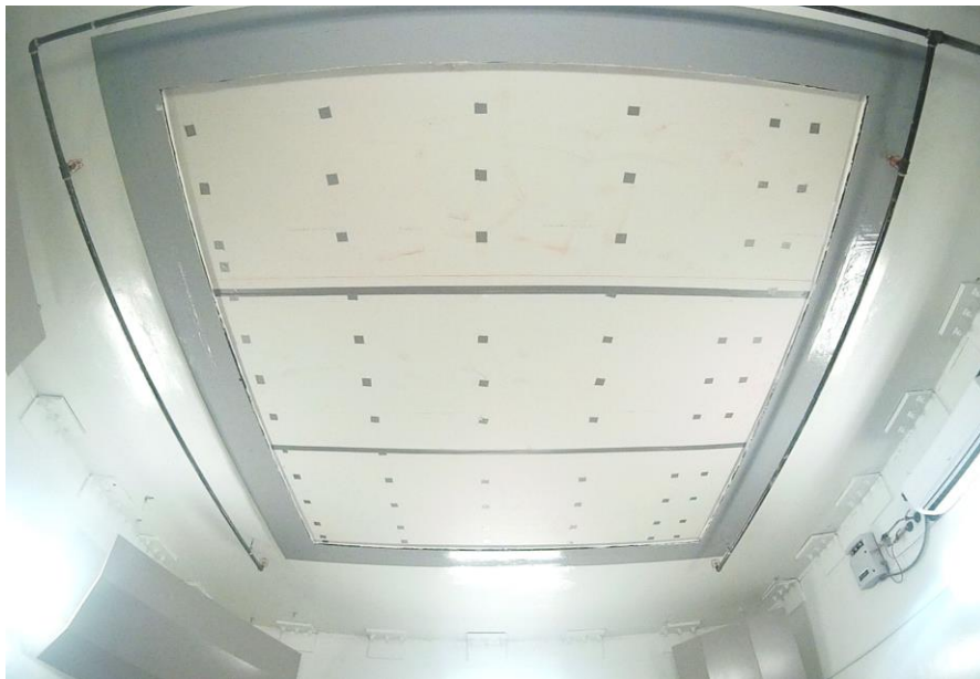
Receive Room View of Test Specimen Installation
