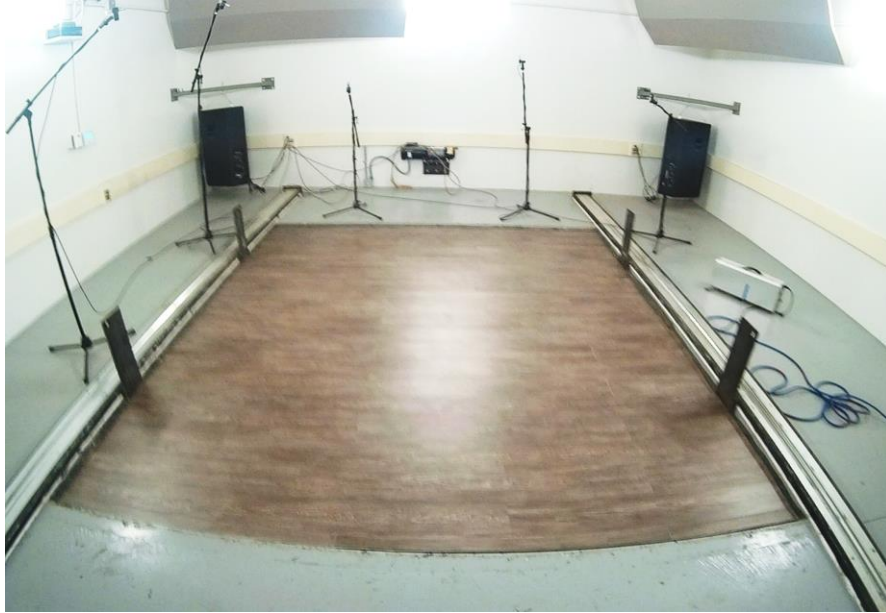
Source Room View of Test Specimen Installation
